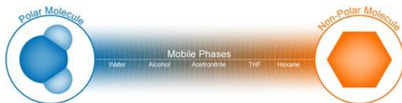
Figure R-1: Mobile Phase Chromatographic Polarity Spectrum
