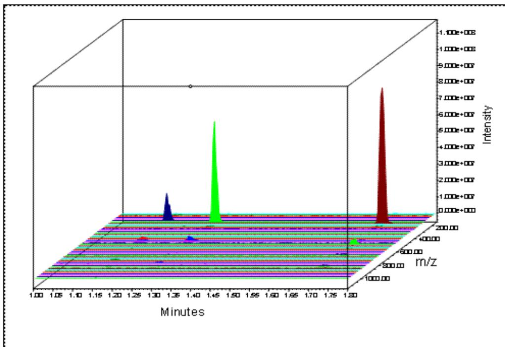
Figure 10: 3 dimensional plot of the same 3 sulfa drugs as in Figure 9, using a mass spectrometer detector
