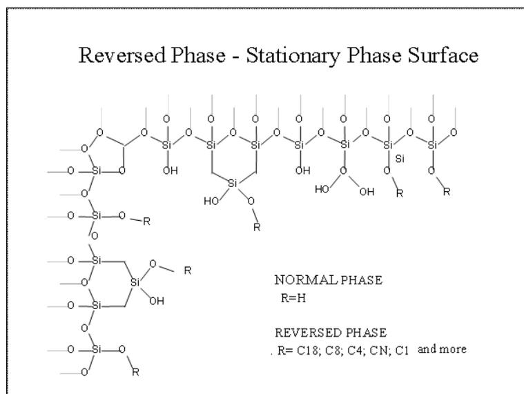
Figure 2: The surface of Reversed Phase stationary phases
