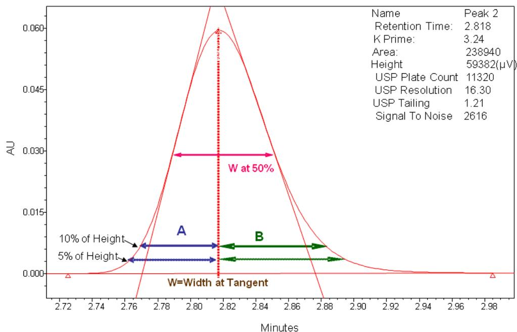
Figure 5: System Suitability measurements on a single peak
