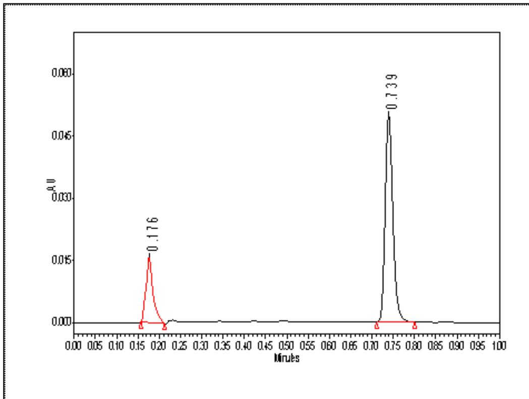
Figure 3: Example of Capacity factor calculation in LC. In this case:  $t_R = 0.739$ ,  $t_0 = 0.17$ , therefore  $k' = (0.739-0.176)/0.176 = 3.20$
