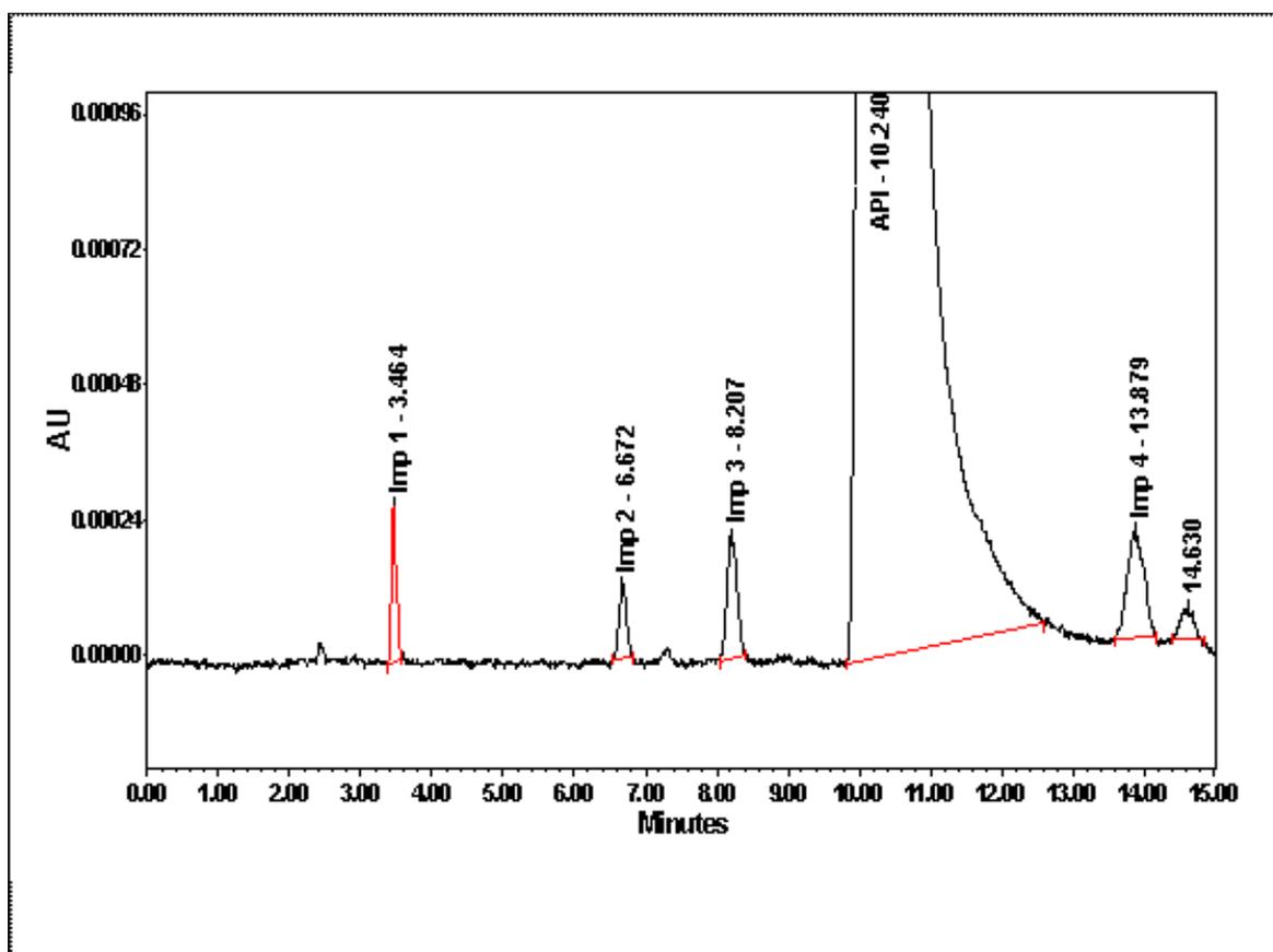
Figure 8: A chromatogram of an API sample at a stability program. Detection: UV at 286 nm, isocratic run (70:30 water:acetonitrile with 0.1% TFA); Flow rate=1 ml/min. Results are shown in Table 2.
