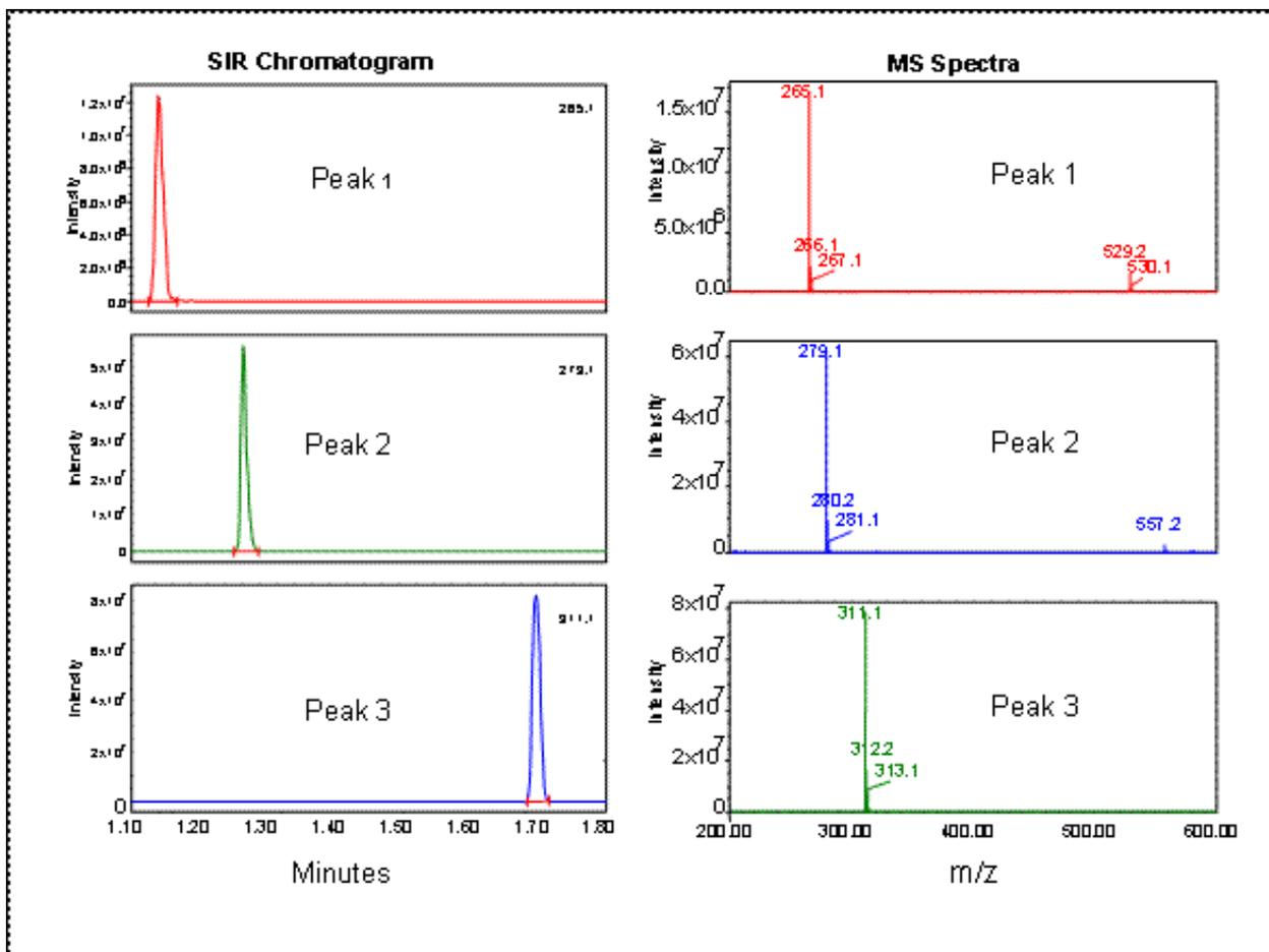
Figure 12: SIR chromatograms of the same sulfa drugs as in Figure 10 and their corresponding mass spectra, obtained by combining spectra across the entire peak.
