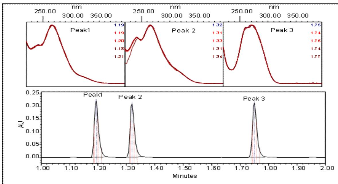
Figure 11: UV chromatogram at 270 nm of three sulfa drugs shown in Figure 9, and a plot of UV Spectra collected from each peak's Apex, Inflection and two offset points, to demonstrate comparison of spectra collected at various points across the peak.
