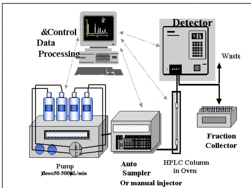
Figure 1: A Scheme of an HPLC System
