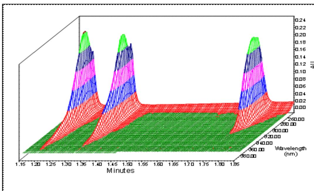
Figure 9: 3 dimensional plot of a chromatographic run of 3 sulfa drugs, using a diode-array detector
