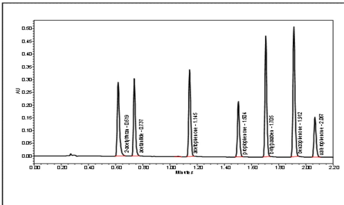
Figure 13: Mixture of alkylphenones injected into Waters' Acquity UPLC using Acquity BEH C18 2.1x50 mm 1.7  $\mu$ m
